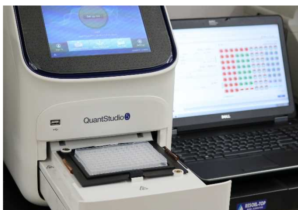
Quantitative PCR instrument
